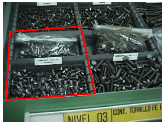
Fig. 6. Reorder point for parts with a 2 bin system design using fit size packages..
